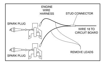
Figure 35. Engine Ground Harness
